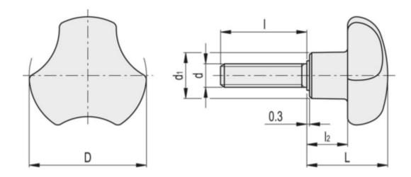
$\begin{array}{lll} D & = 40 \\ d1 & = 16 \\ Dg & = - \\ I2 & = 13.5 \\ L & = 27 \\ L1 & = 20 \\ Weight in (g) = 28 \end{array}$
